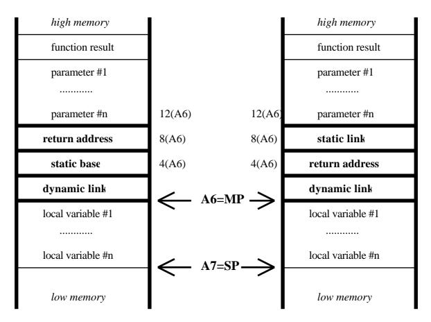
Fig. 4.7: System Stack and Procedure Mark
