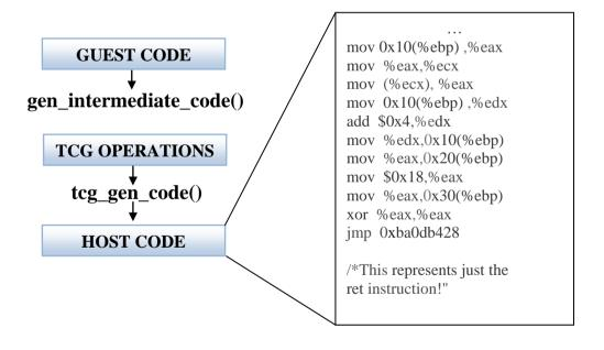
Figure 7.7: Dynamic translation – Showing Generated host Code (shown in assembly for readability)
